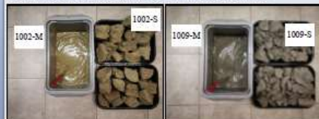
Fig. 1: Natural clay samples, both in two forms: slurry (M) and dried core (S)
